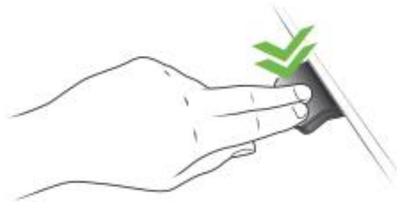
Figure 37: Double-tap to automatically adjust the desk to a favourite position
