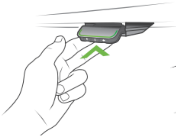
Figure 33: Tilt and hold the DPG1C to drive the desk up
