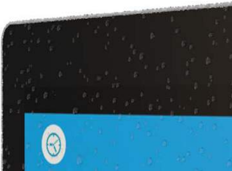
All monitor/AIO front panels are IP65 Rated
